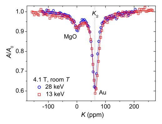
Figure 3.2: Typical high field spectra of  ${}^{8}\text{Li}^{+}$  implanted into 100 nm Au/MgO ( $H_{1} \sim 3 \,\mu\text{T}$ ) showing the large resonance in Au and its Knight shift relative to the resonance in MgO. Each spectrum is fit to two Lorentzians. Reproduced in part from Ref. [212]. Copyright (2008) by the American Physical Society.
