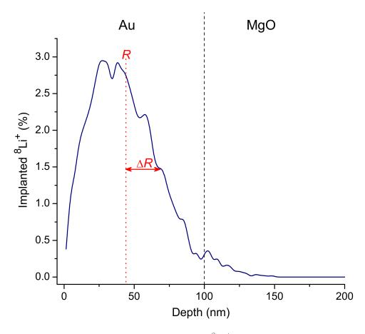
Figure B.1: Stopping profile for 13 keV <sup>8</sup>Li<sup>+</sup> implanted into a 100 nm Au film on MgO. The mean range R = 44 nm, and the range straggling  $\Delta R \sim \pm 25$  nm. The small peaks in the curve are numerical noise due to the relatively small number of particles used in the simulation  $(1 \times 10^4)$ .
