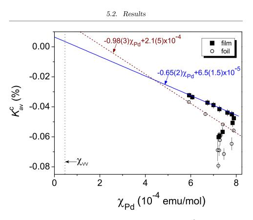
Figure 5.4: Demagnetization-corrected average shifts for <sup>8</sup>Li<sup>+</sup> in the film and foil versus the susceptibility of Pd. At high temperature (small  $\chi_{Pd}$ ),  $K_{av}^c$  is linear with the susceptibility as illustrated by the best-fit lines. The vertical line denotes the van Vleck (orbital) susceptibility of Pd[11].
