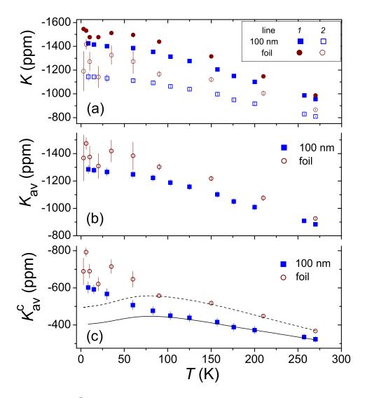
Figure 5.3: <sup>8</sup>Li Knight shifts measured in the 100 nm film and Pd foil (Chapter 4) and as a function of temperature. (a) Raw shifts of the two lines used to fit the Pd signals from both samples, and (b) the average of the shift of the two lines in (a). (c) Average shifts from (b) corrected for the demagnetization using the literature  $\chi_{\rm Pd}$ . The lines indicate the shift values if  $K_{\rm av}^c$  scaled with the susceptibility of Pd for all T (cf. Fig. 5.4).
