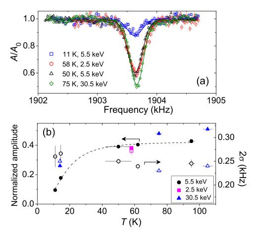
Figure 3.5: Low  $P_{\rm rf} O$  site resonances in Au foil ( $H_0 = 0.3$  T,  $H_1 \sim 0.5 \mu$ T). (a) Representative spectra and single Gaussian fits. (b) Temperature dependence of the amplitudes (filled symbols; left ordinate) and linewidths  $2\sigma$  (open symbols; right ordinate). Below 50 K there is a reduction in the amplitudes as indicated by the dashed line (a guide to the eye) for the low energy data.
