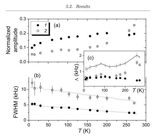
Figure 5.5: Temperature dependence of (a) the normalized amplitudes and (b) the linewidths of the two Lorentzians used in fitting the Pd resonances in the spectra of Fig. 5.1; the dotted lines are guides to the eye. (c) The area  $\Lambda$  of each resonance (FWHM×Normalized amplitude); the continuous line gives their sum.
