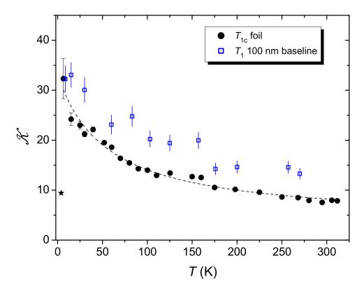
Figure 5.10: Temperature dependence of the Korringa ratio  $\mathcal{K}$  calculated for  $K_{\rm av}^c$  and  $T_{1c}$  or  $T_{1b}$ . The dashed line is a guide to the eye. (\*) denotes the value reported from <sup>105</sup>Pd NMR at 4 K[21].
