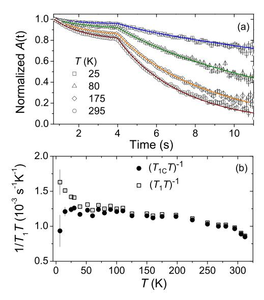
Figure 5.7: (a) Representative spin-lattice relaxation spectra recorded in the Pd foil and associated two component fits using Eqs. (2.7) and (2.8). (b) Temperature dependence of the product  $(T_1T)^{-1}$  for both  $T_1$  and  $T_{1c}$ [the temperature dependence of  $T_1^{-1}$  is shown in Fig. 5.8(b)]. Reproduced in part from Ref. [216]. Copyright (2007) by the American Physical Society.
