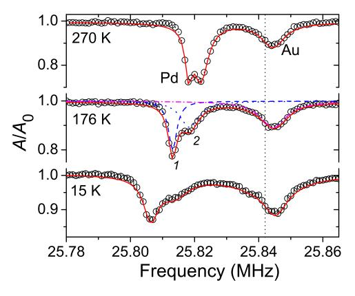
Figure 5.2: Representative spectra from Fig. 5.1 showing the fits to three Lorentzians. The Pd signal is fit to two overlapping lines, denoted 1 and 2, and the Au signal is fit to a single line. The vertical line denotes  $\nu_0$  as determined from the known  $K_S$  in Au (Chapter 3). Reproduced from Ref. [216]. Copyright (2007) by the American Physical Society.
