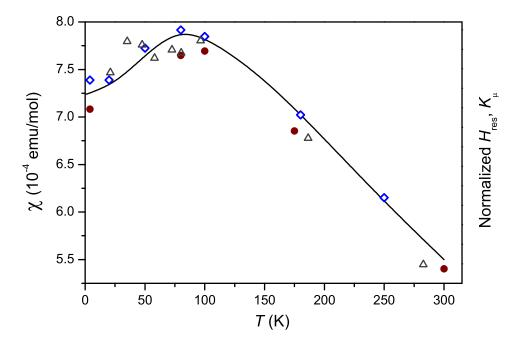
Figure 1.2: Temperature dependence of <sup>105</sup>Pd NMR resonant fields superimposed on the susceptibility of pure Pd: (•), Refs. [14, 21]; ( $\diamond$ ), Ref. [32]. The temperature dependence of the positive muon Knight shift in Pd is also shown ( $\Delta$ ), Ref. [198]. In order to display all the experimental data on the same plot, the NMR resonant fields and muon shifts have been normalized to their respective values at room temperature.
