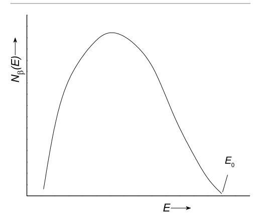
Figure A.1: Example distribution of electron energies in  $\beta$ -decay.  $E_0$  is the maximum energy difference between parent and daughter nuclei; for known  $\beta$ -emitters this ranges between a few keV to about 15 MeV[248].
