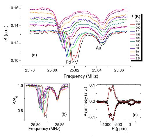
Figure 5.1: (a) Temperature dependence of the <sup>8</sup>Li  $\beta$ -NMR spectra recorded in the Au(10 nm)/Pd(100 nm)/STO film at 4.1 T for  $H_1 \sim 30 \ \mu$ T and  $E_{\rm Li} = 11$  keV. The amplitude of the Pd signal decreases with decreasing T while the amplitude of the Au signal remains constant, as seen in (b) for the normalized spectra. (c) Spectrum from this film ( $H_0 = 6.55$  T,  $H_1 \sim 40$  $\mu$ T, 270 K) in the separate helicity channels.
