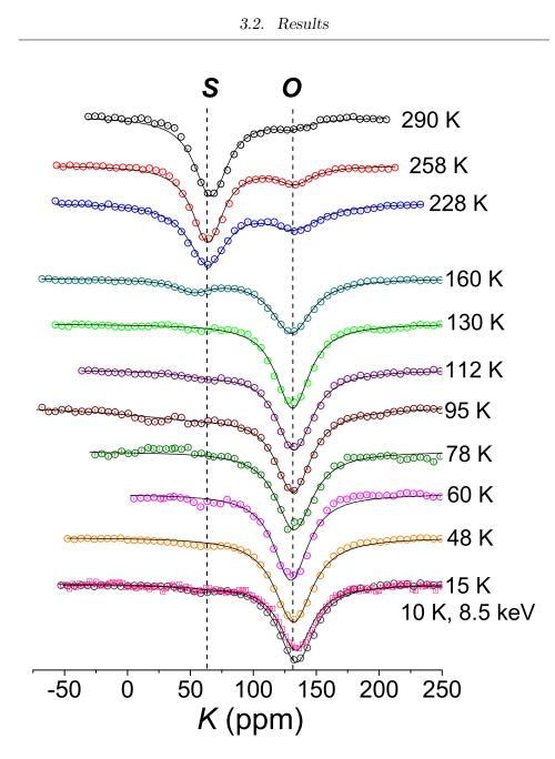
Figure 3.3: Resonance spectra recorded in Au foil for  $H_0 = 3$  T,  $H_1 \sim 5 \mu$ T,  $E_{\rm Li} = 30.5$  keV (circles); and for  $E_{\rm Li} = 8.5$  keV at 10 K (squares). The solid lines are fits using one (T < 150 K) or two Lorentzians (T > 150 K). The abscissa was set using  $K_S$  measured in Fig. 3.2. Reproduced from Ref. [212]. Copyright (2008) by the American Physical Society.
