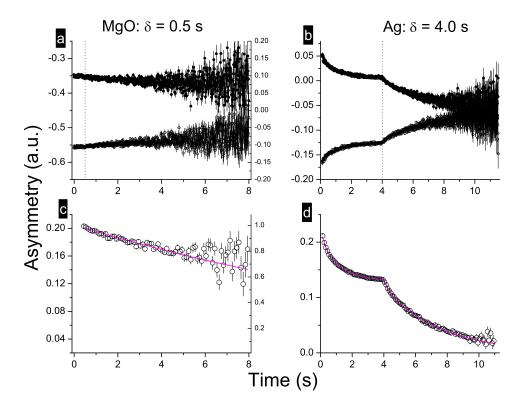
Figure 2.4: Representative spin-lattice relaxation spectra. (a) and (c), Spectrum recorded in a (100) crystal of MgO at room temperature and  $H_0 = 3$  T using  $\delta = 0.5$  s; (b) and (d), spectrum recorded in Ag foil at 250 K and  $H_0 = 15$  mT using  $\delta = 4.0$  s. The top panels show the averaged spectra in the separate helicities; while the bottom panels show the combined spectra after binning.
