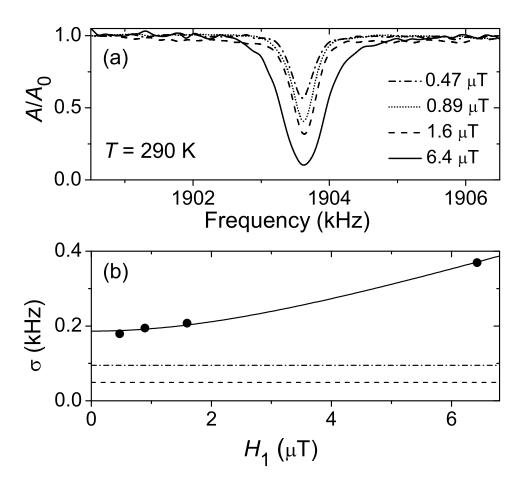
Figure 3.1: (a) Spectra recorded in Au foil ( $H_0 = 0.3$  T,  $E_{\text{Li}} = 30.5$  keV) as a function of the  $P_{\text{rf}}$ , the amplitude of  $H_1$ . (b) Gaussian linewidths  $\sigma$  of the spectra in (a). The intrinsic linewidth  $\sigma_0 = 186(5)$  Hz from the low power limit. The horizontal lines indicate calculated van Vleck linewidths for the undistorted O (dot-dash line) and S (dashed line) sites. Reproduced from Ref. [212]. Copyright (2008) by the American Physical Society.
