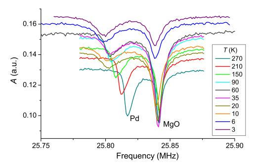
Figure 4.1: Temperature dependence of the <sup>8</sup>Li  $\beta$ -NMR spectrum at 4.1 T ( $H_1 \sim 40 \ \mu$ T) in Pd foil wrapped around crystalline MgO. The spectra have not been offset; the change in baseline asymmetries is due to the increase in spin-lattice relaxation with increasing temperature. Reproduced in part from Ref. [215]. Copyright (2005) by Elsevier B.V.
