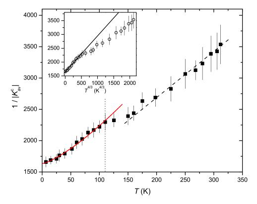
Figure 5.11: Apparent  $T^{4/3}$  dependence of  $1/|K_{\rm av}^c|$  (unitless) below  $T^*$  (red line). The dotted line marks  $T^*$ . For temperatures above 150 K,  $K_{\rm av}^c$  exhibits the same CW behaviour as the host (dashed line; guide to the eye). The inset shows  $1/|K_{\rm av}^c|$  (unitless) plotted against  $T^{4/3}$ .
