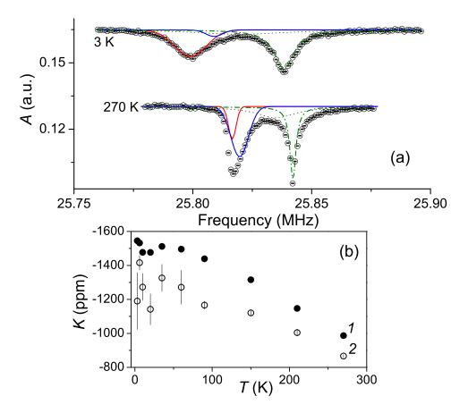
Figure 4.2: (a) Representative fits; the Pd signal is fit using using two overlapping Gaussian lineshapes (solid lines), a single Lorentzian lineshape is used to fit the MgO signal (dash-dot line), and an additional Lorentzian lineshape is added to account for the broad background (dotted line). (b) The resulting K as a function of T for the two Pd lines.
