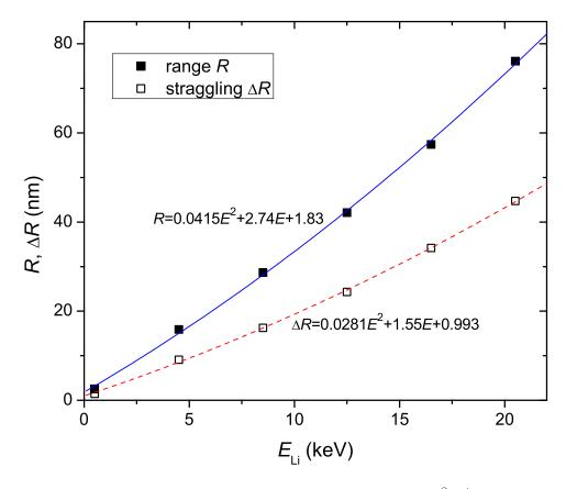
Figure B.3: Mean stopping range R and straggling  $\Delta R$  of <sup>8</sup>Li<sup>+</sup> implanted into Pd as a function of energy as predicted by TRIM.SP. Equations for the associated quadratic interpolation curves are indicated.
