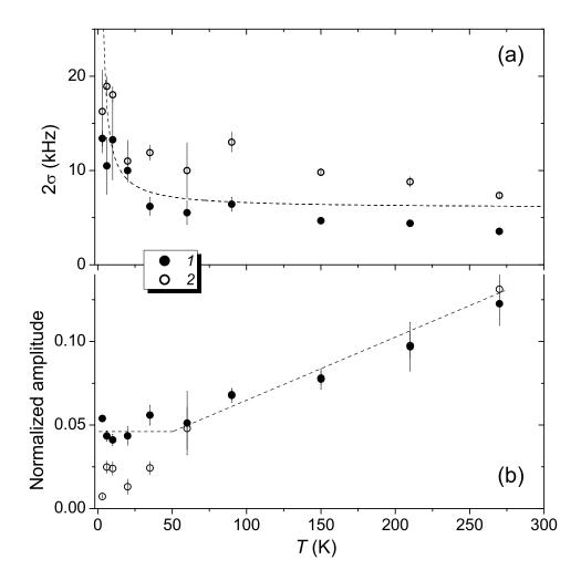
Figure 4.4: (a) Widths of the two Gaussians used in fitting the Pd signal as a function of temperature. The dashed line is an inverse-T function given by (60/T) + 6, and is shown for comparison. (b) Normalized amplitudes of the two Pd lines with temperature; the dashed line is a guide to the eye.
