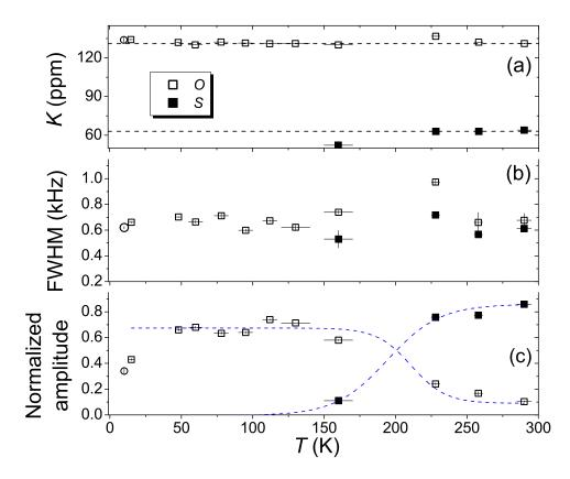
Figure 3.4: Temperature dependence of Knight shifts (a), linewidths (b) and the amplitudes (c), of the 3 T resonances in Au foil from the Lorentzian fits to the data in Fig. 3.3. Circles denote data collected for  $E_{\rm Li} = 8.5$  keV. Reproduced in part from Ref. [212]. Copyright (2008) by the American Physical Society.
