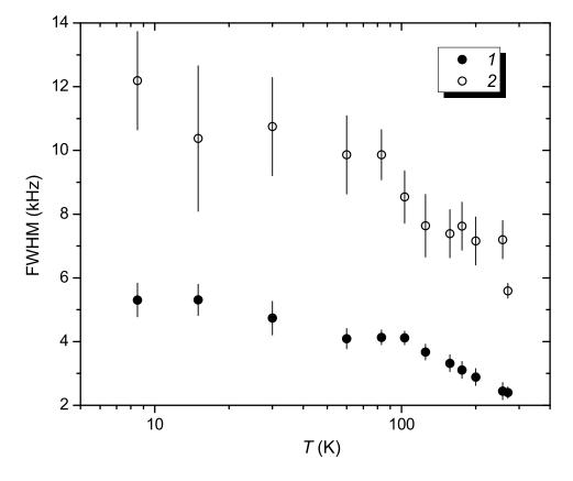
Figure 5.6: Temperature dependence of the linewidths of the two Lorentzians used in fitting the Pd resonances plotted on a semi-logarithmic scale.
