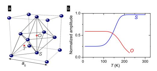
Figure 1.3: (a) Three possible stopping sites of cubic symmetry for an implanted probe in the fcc lattice: the tetrahedral ( $\mathcal{T}$ ) and octahedral (O) intersitial sites, and the substitutional sites (S). (b) Temperature dependence of the resonance amplitudes assigned to <sup>8</sup>Li<sup>+</sup> occupying the S and O sites in a 50 nm Ag film, as reported in Ref. [184].
