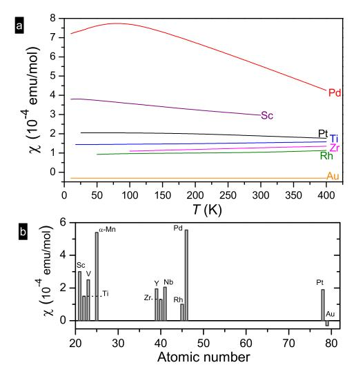
Figure 1.1: (a) Temperature dependence of the suceptibility of selected d metals: Ti and Rh, Ref. [3]; Pd, Refs. [13, 14, 15]; Sc, Refs. [16, 17]; Zr, Refs. [3, 4]; Pt, Ref. [18]; Au, Ref. [1]. (b) Comparison of the *room temperature* susceptibilities of the metals in (a), plus some others with large  $\chi[4]$ .
