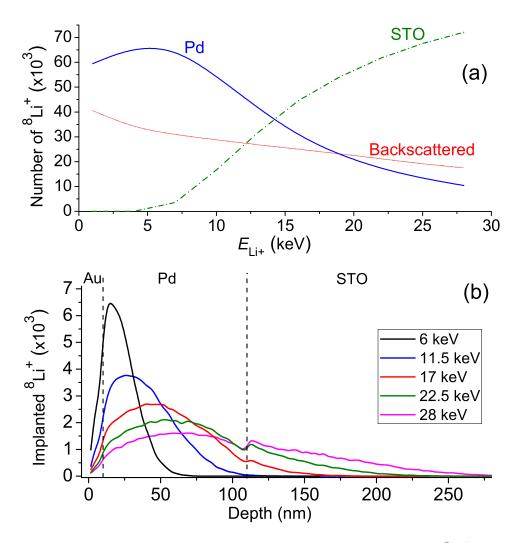
Figure B.2: Examples of results from TRIM.SP simulations of  ${}^{8}\text{Li}^{+}$  implantation into Pd films. (a) Fraction of ions predicted to be implanted into the metal or substrate, and those that are backscattered as a function of ion energy for 50 nm of Pd on STO. (b) Range profiles in Au(10 nm)/Pd(100 nm)/STO for various implantation energies. In both (a) and (b),  $1 \times 10^{5}$  particles were used in the simulations.
