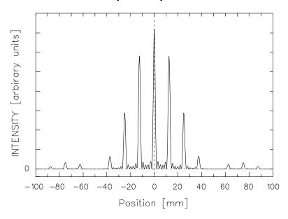
A grating is uniformly illuminated with infrared light of wavelength  $\lambda=1~\mu{\rm m}$  incident normal to the plane of the grating, producing the interference pattern shown at left on a screen 1 m away.
