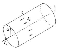
A net current  $I_0$  flows down the solid central conductor and back (in the opposite direction) along the thin outer conductor. The current density  $\vec{J}$  is uniform over the cross-sectional area of the central conductor and the returning current is uniformly distributed over the surface of the outer conducting shell.
