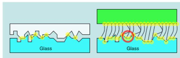
3. The compression only becomes ineffective if the setae are deformed to the point that the spatulae no longer mate with the surface.
