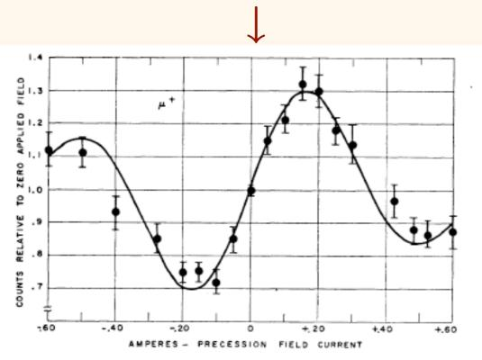
Fig. 2. Variation of gated 3–4 counting rate with magnetizing current. The solid curve is computed from an assumed electron angular distribution  $1-\frac{1}{3}\cos\theta$ , with counter and gate-width resolution folded in.
