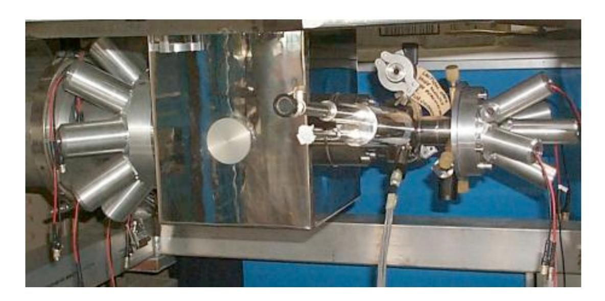
Fields of up to 8 T are now available, requiring a "business end" of the spectrometer only 3 cm in diameter (so that 30-50 MeV decay positron orbits don't "curl up" and miss the detectors) and a time resolution of  $\sim$  150 ps. Muonium precession frequencies of over 2 GHz have been studied.
