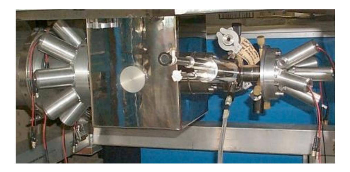
Fields of up to 10 T are now available, requiring a "business end" of the spectrometer < 3 cm in diameter (so that 30-50 MeV decay positron orbits don't "curl up" and miss the detectors) and a time resolution of ~ 150 ps. Muonium precession frequencies of over 2 GHz have been studied.
