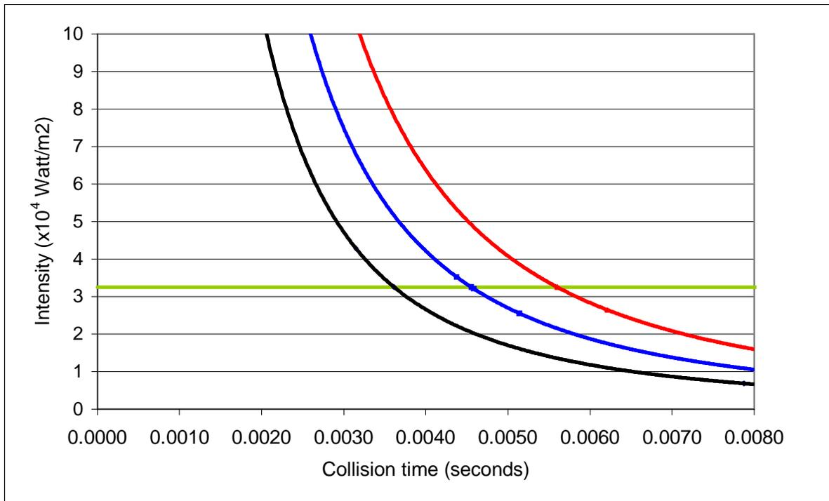
**Figure 4.** Intensities of waves generated by tail slaps from whales of different body length, and the varying collision times at which wave intensity is equal to the fatal intensity.
