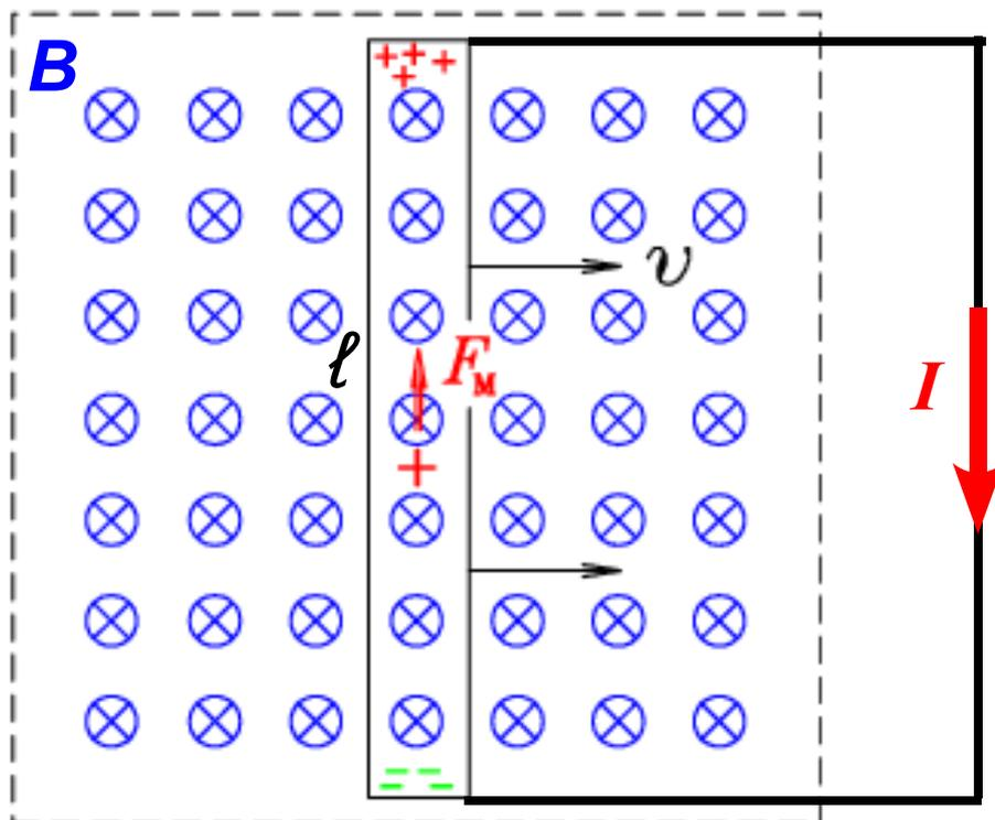
current will flow **clockwise** here, so as to reunite the **+** & **-** charges. This current makes its own magnetic field into the page, and thus **adds** to the net flux through the loop in that direction, which **was decreasing** as the loop was pulled out of the field. So the induced EMF "tries" to make a current flow to counteract the change in flux. (**Lenz's Law**)
