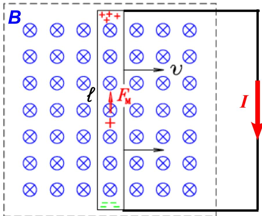
Law is that it applies (and works!) equally in situations that bear no resemblance to this example. If there is **no physical motion** at all, but only a change in the **strength** of the magnetic field, we still get an induced EMF according to the same equation. This accounts for the enormous impact of "electric power" on the modern world. It also leads to our understanding of the nature of light itself.
