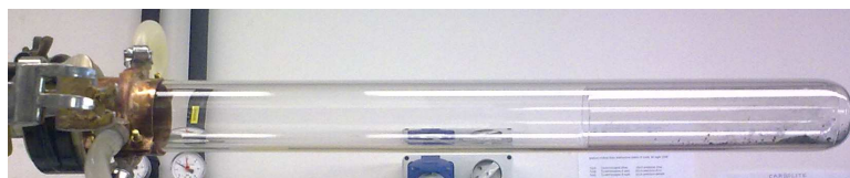
(a). The GO powder is loaded inside a vial for the thermal exfoliation treatment.
