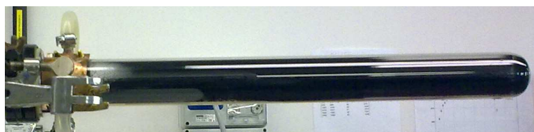
(b). The expansion of graphite to graphene leads to a huge increase in volume.
