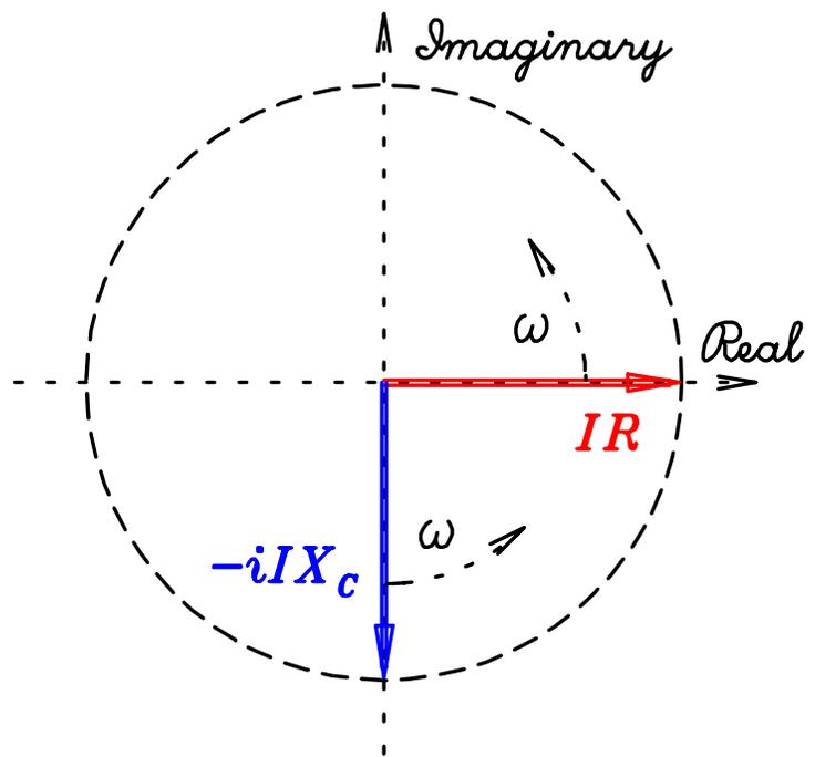
The voltage across the *capacitor lags behind* that across the resistor by an angle of  $\pi/2$ .
